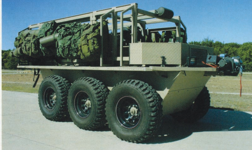
SMSS robot vehicle is sized for use by infantry squads and special forces teams, and has all-terrain capabilities.
